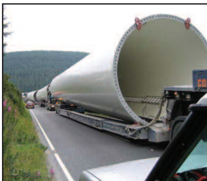
A convoy carrying the body of a wind turbine makes its way to an already prepared foundation.
